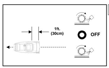
Release intermittent setting or turn off continuous setting on brush/spray switch approximately 1 foot before ending cleaning pass.
